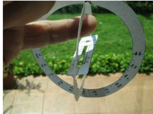
While balancing on your finger/thread, rotate the ring until sunlight from the square hole, made by the mask, shines on the outer hour ring.
