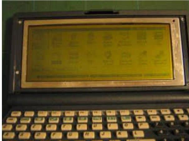
Now place the plastic bezel back to its original position and press down gently. The bezel would hold the polarizer in place.
