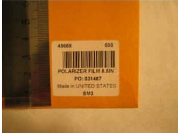
Cut out a rectangle 2" x 5" from the sheet. ie: As the orientation is important, with the long size placed horizontally, make a vertical cut. Use a pair of scissors, to snip of 1mm from the longest side. To the longest side would thus be 5"-1mm so that it would fit within the metal frame of the screen.
