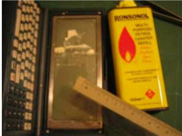
Remove these shavings with tissues from time to time. When almost all of the film and glue stains have been removed, polish the glass with a pad of tissue soaked in lighter fluid. That would remove the rest of the residue on the screen.
